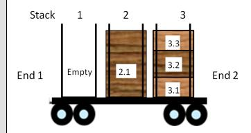
Transport unit identifier for the RailCar with 3 loading stacks is 917400000019. Loading stack number 1 is empty.
