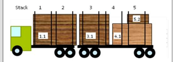
Transport unit identifier for the DrawBarCombination with 5 loading stacks is ABC222. The transport unit is loaded with long logs taken up more space than one loading stack. The Identifier for the first log pile is ABC222\_1.1, followed by log pile ABC222\_3.1, ABC222\_4.1 and ABC222\_5.2.
