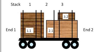
Transport unit identifier for the RailCar with 3 loading stacks is 917400000019. The transport unit is loaded with long logs taken up more space than one loading stack. The Identifier for the first log pile is 917400000019\_1.1, followed by log pile 917400000019\_2.1 and 917400000019\_3.2.
