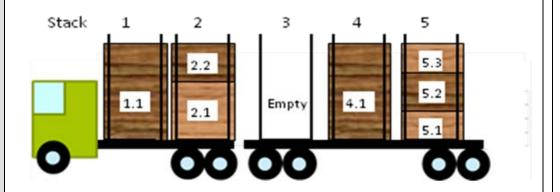
Transport unit identifier for the DrawBarCombination with 5 loading stacks is ABC222. Loading stack number 3 is empty.
